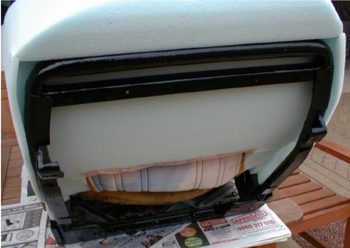
(12) First job is to place the foam base over the frame to check for fit.
